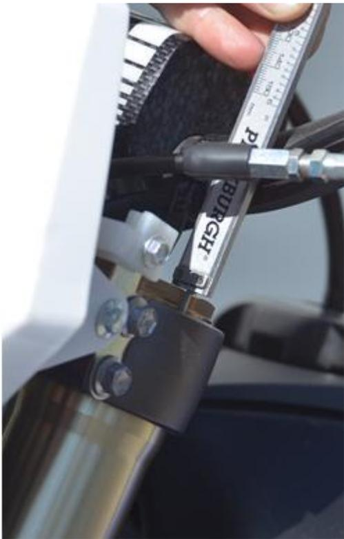
2- Check that both of the forks are installed at the same height. Start at factory settings.
