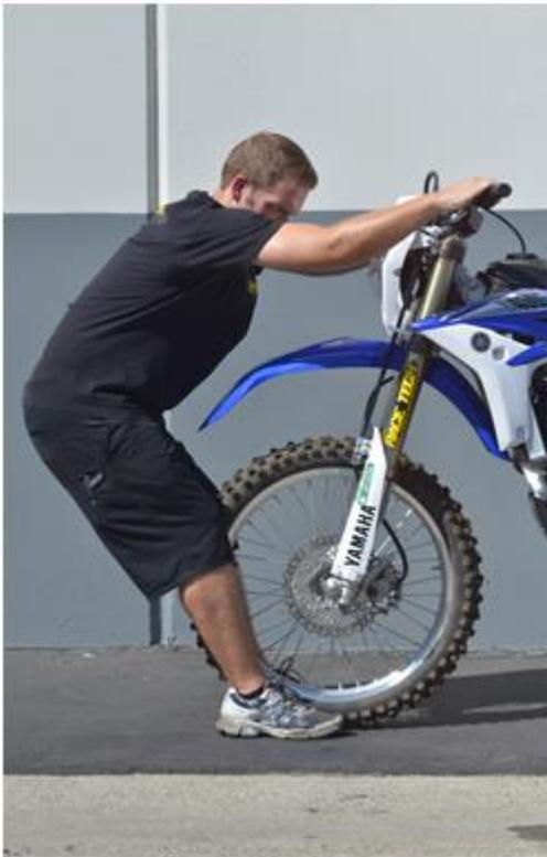
17- Another way to align the fork tubes is to compress the front a few times while holding the front brake.
