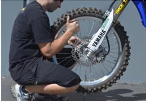
10- Put the wheel into position and make sure the brake disk easily slides into the brake caliper between the pads.
