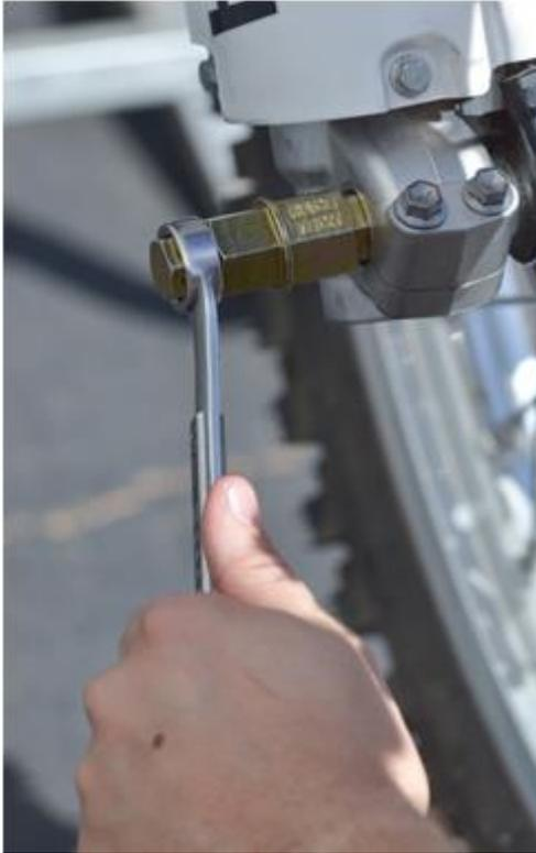
13- Using the RT Axle Tool (TFHD 1724) hold the axle in place. You can also hold the axle by pinching it with the large diameter non-threaded (no nut) axle clamp (in this case the right side - shown) as well but you **MUST** make sure you loosen the axle clamp to do the next step - **THIS IS THE NUMBER ONE ERROR PEOPLE MAKE.**
