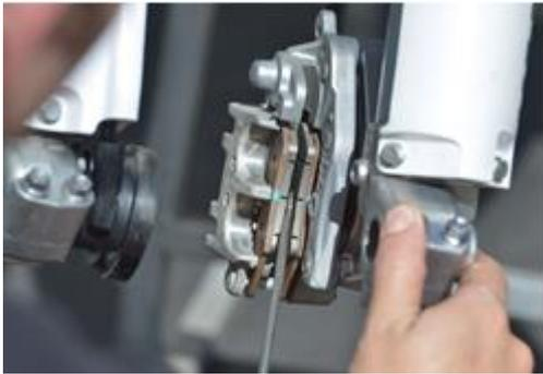
8- Check that the brake pads are separated for ease of wheel installation.
