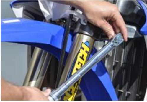
3- Torque the pinch bolts down to OEM specifications (usually 16 ft-lbs for the top, 14 ft-lbs for the bottom - but please check).
