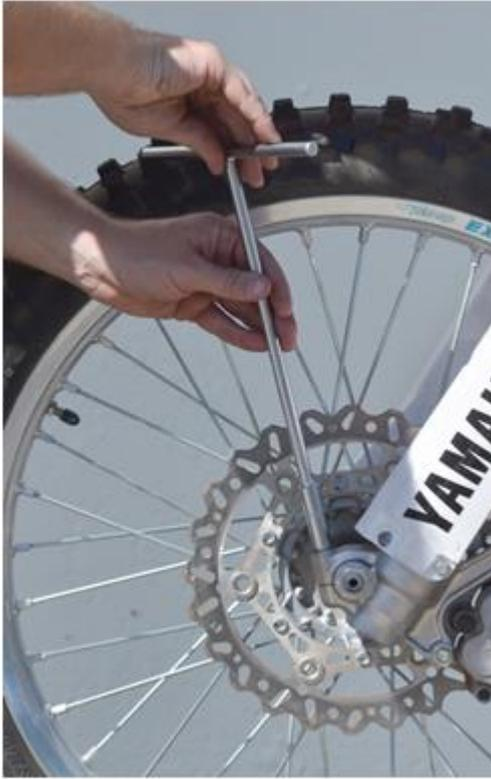
18- Once the forks are properly aligned, tighten the axle pinch bolts.
