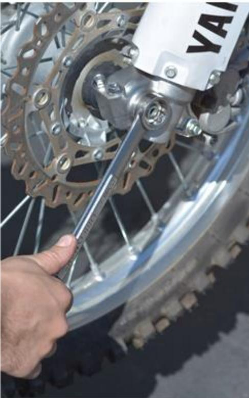
14- Tighten the axle nut.
