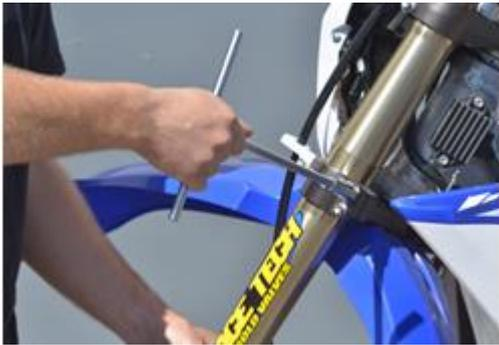
1- Slide the forks through the triple clamps and lightly tighten the pinch bolts.
