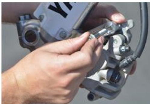
6- Insert the brake calipers bolts...
