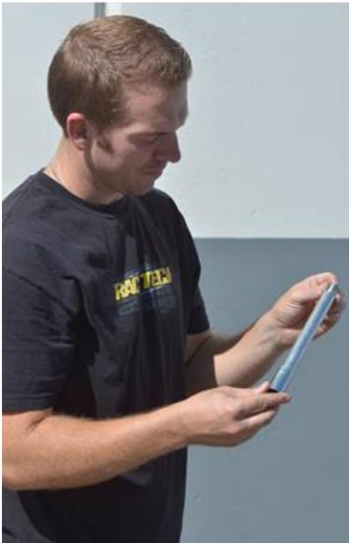
9- Check the axle for any burrs or lips particularly at the transition where it steps up to the largest diameter (this is common and is often the source of fork bind). File these burrs if necessary.
